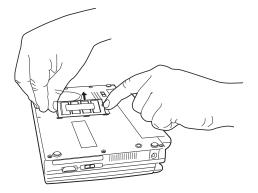
Sample removing the memory module
